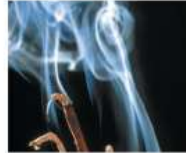
12.20 The flow of smoke rising from these incense sticks is laminar up to a certain point, and then becomes turbulent.
