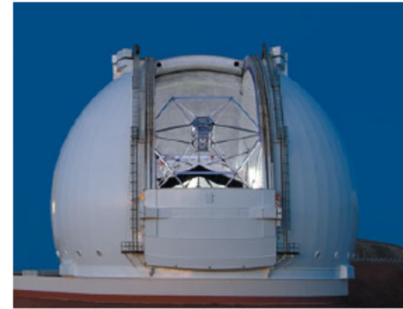
FIGURE 25-22 A concave mirror can be used as the objective of an astronomical telescope. Arrangement (a) is called the Newtonian focus, and (b) the Cassegrainian focus. Other arrangements are also possible. (c) The 200-inch (mirror diameter) Hale telescope on Palomar Mountain in California. (d) The 10-meter Keck telescope on Mauna Kea, Hawaii. The Keck combines thirty-six 1.8-meter six-sided mirrors into the equivalent of a very large single reflector, 10 m in diameter.
