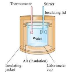
The instrument to the left is a calorimeter, which makes quantitative measurements of heat exchange. A sample is heated to a well-measured high temperature, plunged into the water, and the equilibrium temperature measured. This gives the specific heat of the sample.
