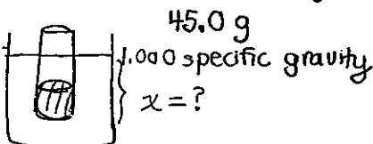
$$\frac{x}{25.0 \text{ cm}} = \frac{\rho_{\text{tube}}}{\rho_F} = \frac{45.0 \text{ g} / (25 \times 2 \text{ cm}^3)}{1.0 \text{ g/cm}^3}$$
