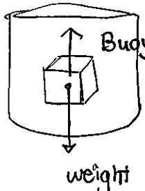
Buoyant force = weight of displaced water
