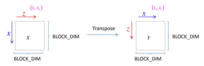
$zIndex = t_1 \cdot BLOCK \_DIM + threadIdx.x$  $xIndex = t_2 \cdot BLOCK \_DIM + threadIdx.y$
