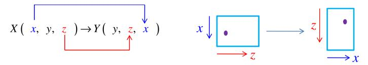
The simplest way is (1) use 2D grid to represent (x, z) slice and do transpose operation along y
