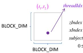
$\begin{aligned} zIndex &= t_1 \cdot BLOCK \_DIM + threadIdx.x \\ xIndex &= t_2 \cdot BLOCK \_DIM + threadIdx.y \\ subject & \left(zIndex, xIndex\right) \equiv \left(k-1, i-1\right) \text{ since } X\left(1:n_1, 1:n_2, 1:n_3\right) \\ 0 &\leq xIndex < n_1 \ , \quad 0 \leq zIndex < n_3 \end{aligned}$
