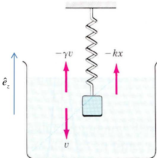
$$\vec{F} = \vec{F}_{spring} + \vec{F}_{resistance} \quad (\text{ignore buoyancy 浮力})$$
