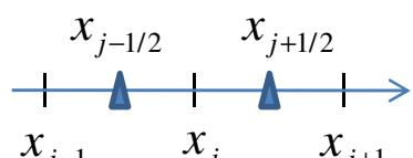
$$\frac{d^2 f}{dx^2}(x) = \frac{\frac{df}{dx}(x_{j+1/2}) - \frac{df}{dx}(x_{j-1/2})}{h} - \frac{h^2}{6} \left( \frac{df}{dx} \right)^{(3)} + O(h^4) \text{ short-stencil}$$
