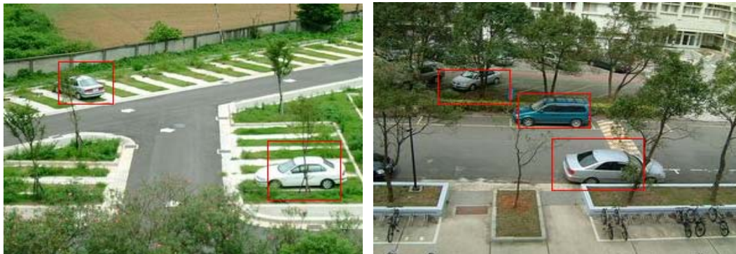
Fig. 30: Results of vehicle detection when occlusions happened.
