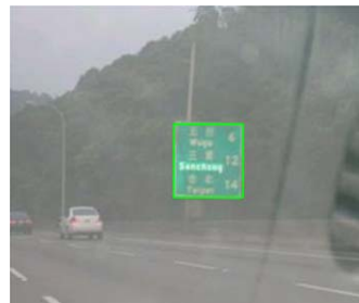
Fig. 37: Results of road sign detection when low contrast video frames were handled.
