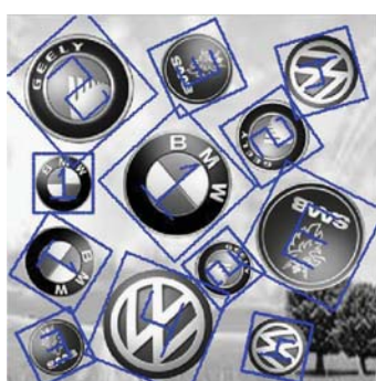
Fig. 11. Result of template matching for 4 templates with RST variations ( K=0.3 ).
