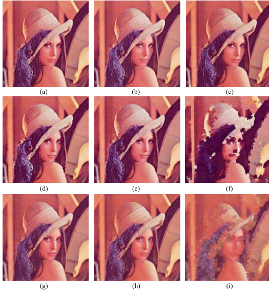
Fig. 7. Opening and closing operations. (a)Original image, (b) M-ordering opening, (c) M-ordering closing, (d) HC-ordering opening (SE=3, without ARCS), (e) HC-ordering opening (SE=3, with ARCS), (f) HC-ordering opening (SE=10, with ARCS), (g) HC-ordering closing (SE=3, without ARCS), (h) HC-ordering closing (SE=3, with ARCS), and (i) HC-ordering closing (SE=10, with ARCS).
